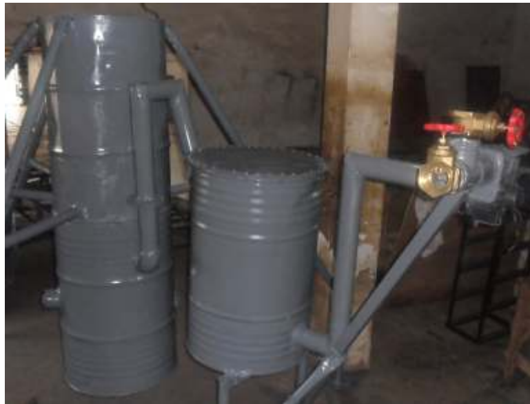
Quintas Downdraft Gasifier for Syngas Generation
