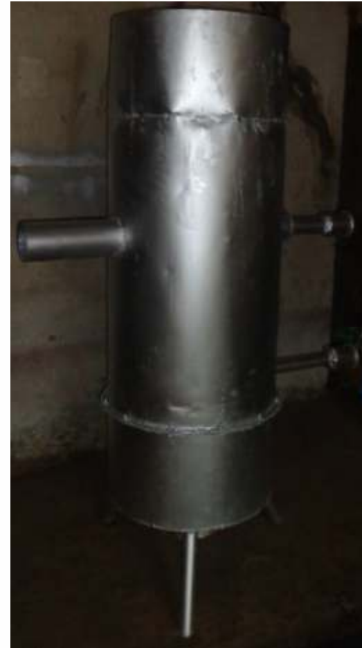
250kW Quintas Gasifier with embedded combustor
